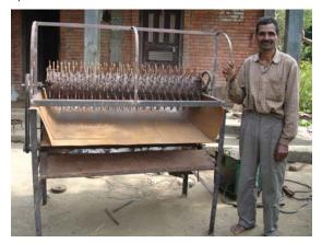
He is trying to improve the speed of the fan to reduce vibration. The cost of making a thresher is Rs 30,000. To date, a farmer from Fulbari VDC has demanded such a thresher and Mr. Neupane is making one for him.
