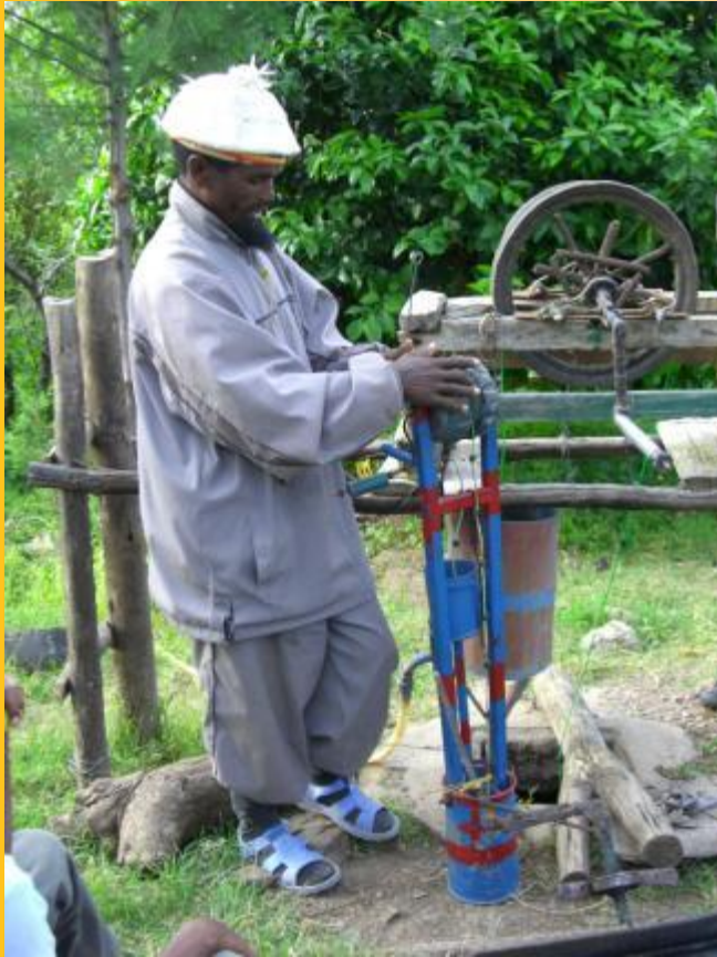
Ethiopian farmer innovator developed water-lifting devices working with local blacksmith
